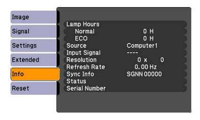
**Note:** The lamp usage timer does not register any hours until you have used the lamp for at least 10 hours. Available settings depend on the current input source.
